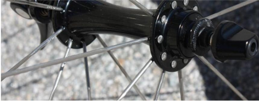
Minimal hubs come standard with steel bearings. FLO offers a \$100 upgrade to ceramic bearings with proceeds going to the company's Bike For a Kid charity.
