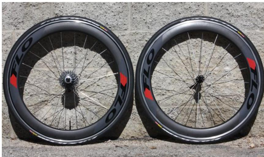
Rather than simply building a wheel line by picking some readily available carbon rims from an Asian production catalog, FLO developed their own products using CFD (Computational Fluid Dynamics) software and a healthy amount of testing at the A2 wind tunnel. The "60" model is 60mm deep and measures 28mm wide. It sells for \$898 for the set and includes quick release skewers and a 2-year manufacturer's warranty. Custom decals are also on offer.
